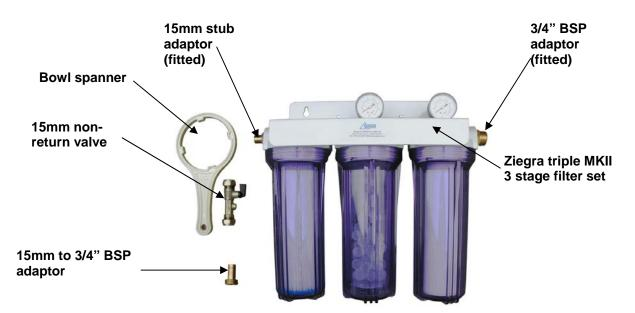
You will need to supply a 15mm copper or plastic water supply terminating in a 3/4" BSP fitting and a food quality water hose for the water inlet side. Alternatively the 15mm supply can be plumbed straight into the inlet compression fitting of the non-return valve. You will need another food quality water hose to connect the outlet of the filter to the machine. UBE1.500 and above have a 1/2" BSP water inlet, so for these machines you will also need a 1/2" to 3/4" adaptor bush.
